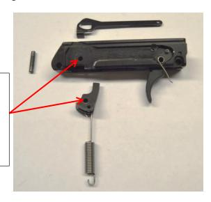
Reinstall the trigger bar making sure the small hole on the transfer bar goes over the small post on the trigger pivot block.
