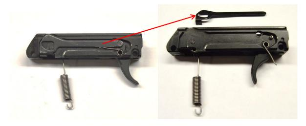
Push the hammer pivot pin out with a small punch and remove the hammer from the internal metal frame. This should easily slide out. Set the trigger bar and hammer pivot pin aside.
