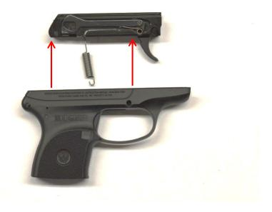
Step 4a: Installation of the hammer spring:
