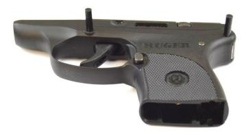
Step 6: Install hammer spring pin, hook on hammer spring, and reinstall polymer grip cap:
