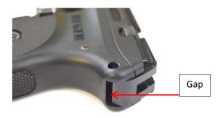
While holding the internal metal frame downward into the polymer grip, insert a small flat head screwdriver or pick into the rear of this gap. Lift the hammer reset lever (shown on next page) with the tip of the screwdriver and push this lever forward. Once this lever is forward (and you are still holding the metal frame downward), remove the screwdriver. The internal metal frame should fully seat into
