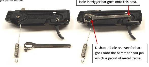
Rotate the arm of the Fort Wayne Tactical LLC trigger reset spring counter-clockwise and hook it under the transfer bar. The transfer bar has a small groove that the arm of this spring will rest on.
