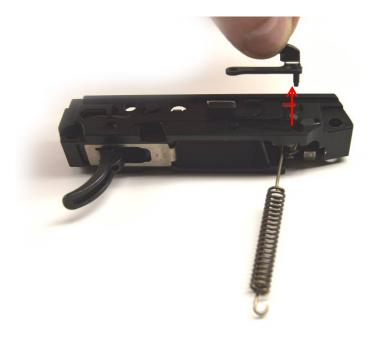
Using a pick, pull the arm of the stock trigger reset spring out from under the trigger bar. The stock trigger reset spring will NOT be able to be removed from the metal frame at this time.
