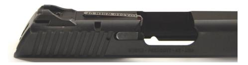
Using a brass faced hammer, tap the roll pin partially into the cross hole on the slide until it just starts to engage the loaded chamber indicator. At this point you'll want to verify that the loaded chamber indicator pivots freely on the roll pin.
