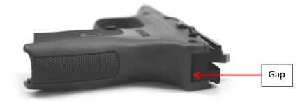
While holding the internal metal frame downward into the polymer grip, insert a small flat head screwdriver or pick into the rear of this gap. Lift the hammer reset lever (shown on next page) with the tip of the screwdriver and push this lever forward. Once this lever is forward (and you are still holding the metal frame downward), remove the screwdriver. The internal metal frame should fully seat into
