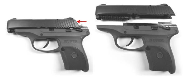
Remove the recoil spring and guide rod from the slide.
