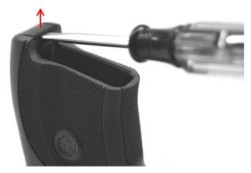
Step 3: Removal of the metal internal frame from the polymer grip:
