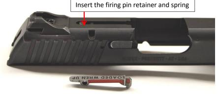
Insert the loaded chamber indicator into the top of the slide and line up the pivot hole on the loaded chamber indicator with the cross hole on the slide.
