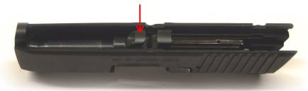
Insert the guide rod and recoil spring into the slide. Make sure the back of the guide rod seats on the notch on the back of the guide rod.
