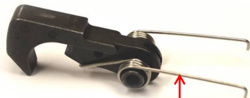
Install FWT hammer spring
