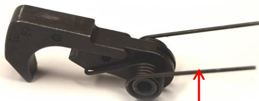
Remove mil spec hammer spring
